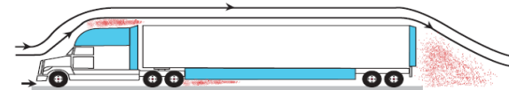
B: A tractor-trailer with aerodynamic devices installed produces less drag (shown as shaded area)
